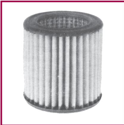
and long life at low pressure drop is required. Performance is better than 98% efficiency on particles of 3 micron mean diameter, over 99% efficiency on 5 micron mean particles, and virtually 100% efficiency on 10 micron particles and larger. The polyester media element comes with a wrap around prefilter providing extended service life.
