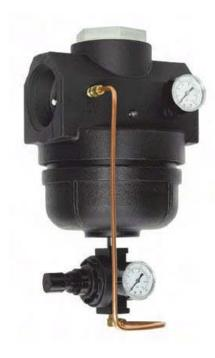
These pilot operated regulators utilize a small auxiliary regulator to supply the required system pressure to a large diaphragm located on the main line valve that regulates the system pressure. A small change in downstream pressure can effect a large change in the pressure applied to the main regulator diaphragm. The main idea behind the pilot operated pressure regulator valve is the need to open or close the main pressure regulator valve very fast by using additional pressure regulator valve.
