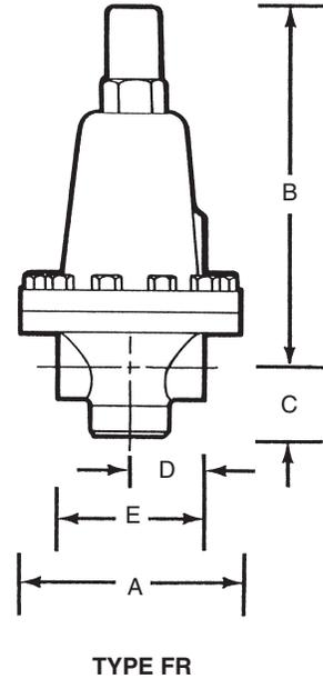
FRM, FRM-2, FRM-C DIAPHRAGM TYPE MINIATURE BACK PRESSURE VALVES
