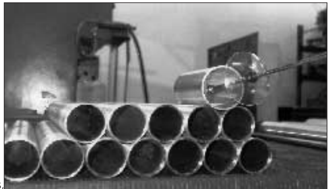
The picture shows blow-out of cylindrical pipe. An Silvent 910 nozzle has been mounted on a Silvent blowing gun fitted with a safety shield.
