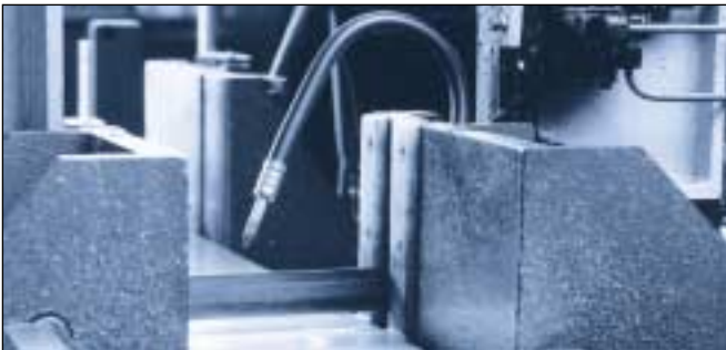
The picture shows a flexblow hose keeping a crosscut saw clean.
