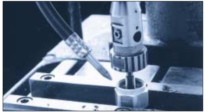
A SILVENT 640 being used for cooling and cleaning in a tapping operation.
