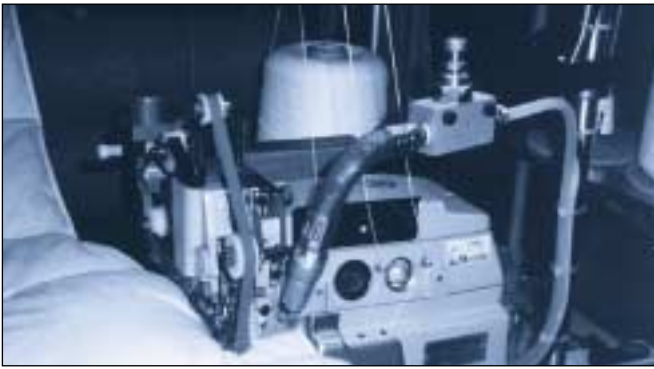
Textile industry. A SILVENT 220 is used to keep the machine clean and avoid stoppage. Previously, a 4 mm open pipe was used. Switching to the 220 cut the noise level in half and reduced air consumption by 36%.
