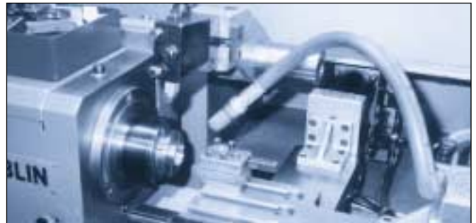
A flexblow hose and a SILVENT nozzle - a very quiet and efficient combination for turning operations.
