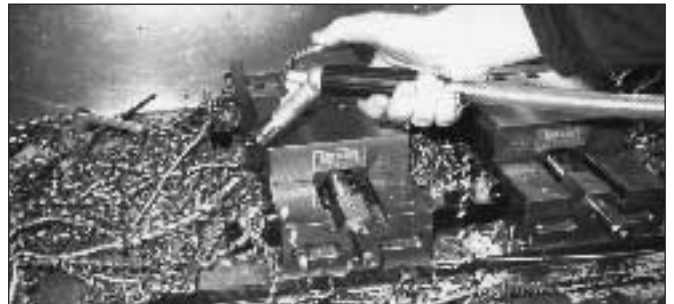
The picture shows blow-off of long, troublesome turnings using the Silvent 755 - a demanding job ordinary blowing guns are incapable of handling.
