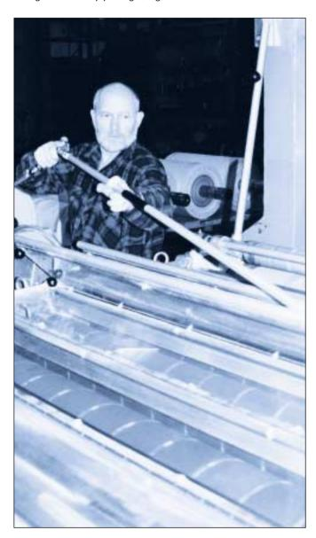
When manufacturing fabric the machines' rollers must be blown clean frequently. This picture illustrates how a 753-S gun with a 1500 mm (59") extension effectively reaches throughout the machine.
