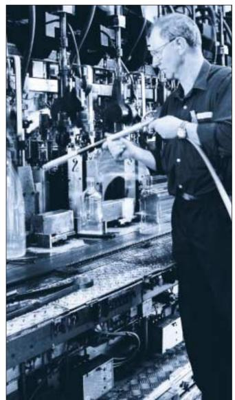
REXAM glassworks in Sweden produces the world famous "Absolut Vodka" bottle. The company uses both Silvent's air guns and fixed nozzle installations to increase compressed air safety and to save air in the plant. The picture shows how a 755-S-500 is used to dislodge molten glass from the molds in connection with stoppage.
