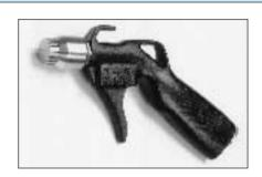
The Silvent 572 is supplied with a stainless steel nozzle (703), instead of the standard Silvent 501 nozzle in zinc (2120). It is used in applications where the nozzle is exposed to heavy mechanical wear or where increased blowing force is desired. This nozzle provides twice the blowing force of Silvent's standard blowing gun, the 501.
