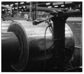
The picture shows a blow-off station for plastic pipe. Silvent 407 nozzle is mounted on a pneumatic rotor arm. The arm is automatically regulated and moves to the opening of the pipe to blow out the long pieces.
