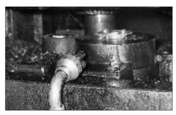
In this application for ejecting parts from a press, a noise level reduction of more than 50% was attained when open pipe was replaced by the Silvent 404.
