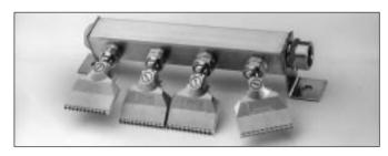
The picture shows a custom air knife with both flow regulation and adjustable swivel joints. These options allow optimization of the blowing force as well as the blowing angle. This particular knife is fitted with four 973F nozzles and four swivel joints (PSK 14) together with mounting brackets (3372).
