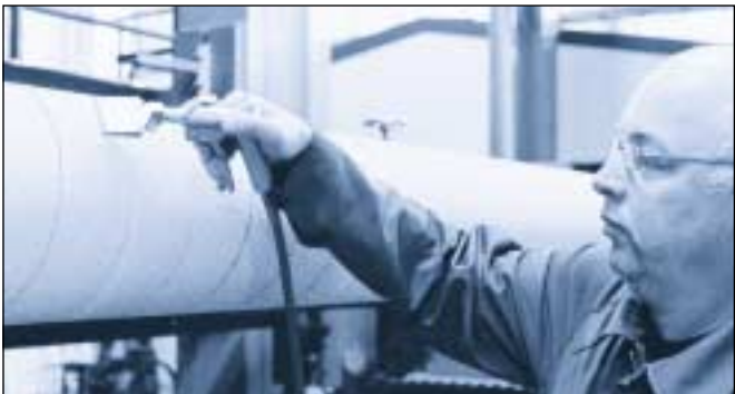
The picture shows an Silvent 2973 efficiently cleaning a large roller at a paper mill. The broad and powerful air cone generated by the flat nozzle does the job three times faster than a conventional air gun.
