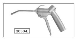
SILVENT 2050-L with a Laval nozzle is an alternative to the stainless steel nozzle described above. The Laval hole in the center of the nozzle provides excellent cleaning properties. Suitable for applications where exposure to mechanical wear is not as great as environments requiring 2050-S. Patented.
