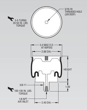
NOTE: The dotted line on the static data chart shows the force capabilities of the 1M1A-1 when attaching an additional 0.5 inch pedestal, provided by the customer, to the base of the air spring. If an additional pedestal is not used, the air spring will behave as the solid line depicts. Without a pedestal the rubber part will contact the ground at the height of 2.1 inches and could cause the rubber part to wear prematurely.
