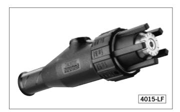
The introduction of the Silvent 4000 constitutes an entirely new concept within blowing technology. Silvent has succeeded in combining highly concentrated blowing force with an easily maneuverable valve construction and low sound level. The nozzle has a patented design with a Laval orifice in its center surrounded by a ring of slots, providing a low-turbulence air stream that means a low sound level and allowing maximum utilization of the energy of the core stream.
