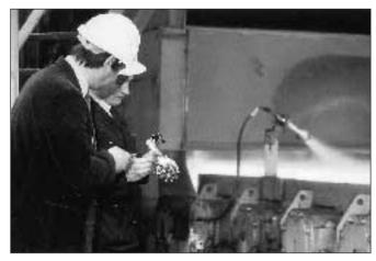
The Silvent 1200 series has solved problems with water and scoria on the hot strip at British Steel. Scale particles and water are effectively swept away as the steel passes the air stream. The open pipe blowing formerly used failed to clean the steel.
