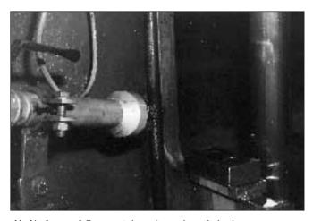
Alu-Norf, one of Germany's largest recyclers of aluminum, uses many different types of Silvent blowing nozzles in their production. Here is one application where a Silvent 1207 is used for blow-off of emulsion in the aluminum making process.
