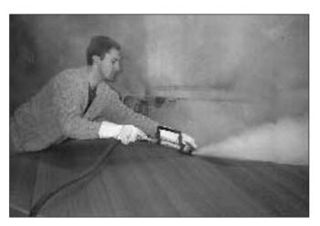
In this application a Silvent 1204 is used to blow hot steam - an unusual application where Silvent helped solve a production problem involving the removal of sticky tape from exclusive veneer. Using the Silvent 1204 lowered the noise level by 50% and virtually eliminated their worst noise problem.
