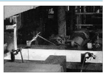
British Steel Corporation is a steady user of Silvent products. The picture above shows how the Silvent 1212 is used to sweep away scale and water from the surface of the steel.
