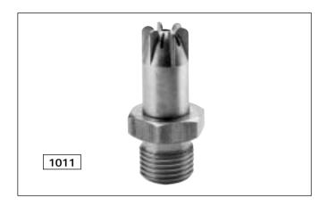
Silvent 1011 is a stainless steel Laval nozzle. A concentrated jet of air traveling at supersonic speed is created through the Laval hole in the center of the nozzle. Around the Laval hole there are a number of diverging slots that generate a powerful, quiet and laminar air stream. This combination utilizes the compressed air optimally. The noise level is cut in half and air consumption is reduced drastically, while efficiency is maintained in comparison with "open pipe blowing".
