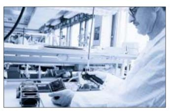
Hasselblad's world famous camera housings are blown clean with high precision and a minimum of compressed air. This is possible thanks to the unique valve design of the 007 grip in combination with a small Micronozzle.
