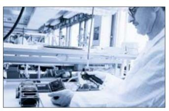
Hasselblad's world famous camera housings are blown clean with high precision and a minimum of compressed air. This is possible thanks to the unique valve design of the 007 grip in combination with a small Micronozzle.
