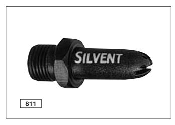
Silvent 811P is a "PEEK" nozzle with a central orifice that can be used in aggressive chemical environments, withstand corrosive cutting fluids and manage temperatures of up to 260° C (500° F). Connection thread 1/8". Additional technical specifications are provided in the table below. Fully meets the EU Machine Directive's noise limitation requirements and OSHA's safety regulations.
