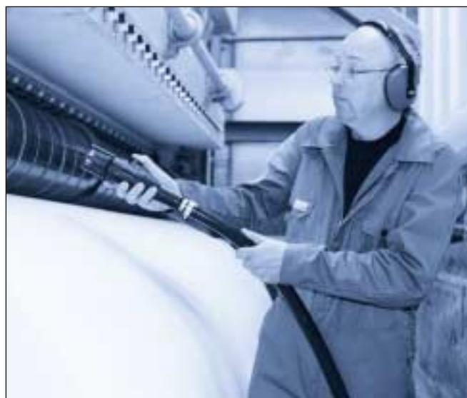
An Silvent 4015-L with "dead man's grip" is used to safely clean a roller. Dead man's grip assures that the valve will close immediately if the operator should drop the grip.
