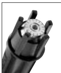
Silvent 4115 has a stainless steel Laval nozzle that provides unique blowing characteristics. The central stream of air is generated by a Laval nozzle which converts all of the energy stored in the compressed air into kinetic energy without allowing the air jet to expand laterally after it has passed through the nozzle. Patented. **Fully meets the EU Machine Directive's noise limitation requirements and OSHA's safety regulations.**
