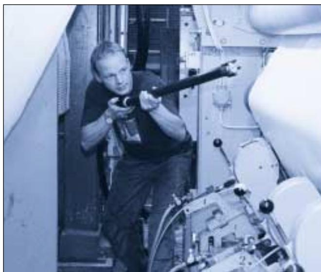
This picture shows a cleaning application at a paper mill. A 4015-L-1000 is used to provide the operator with a more ergonomically correct working posture while allowing him to reach deep within the machine.
