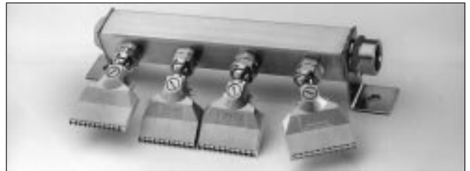
The picture shows a custom air knife with both flow regulation and adjustable swivel joints. These options allow optimization of the blowing force as well as the blowing angle. This particular knife is fitted with four 973F nozzles and four swivel joints (PSK 14) together with mounting brackets (3372).
