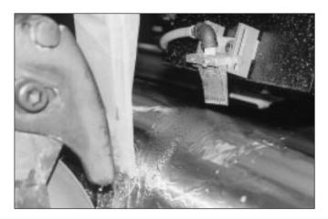
Optimal Dimensions of Montana, USA, uses Silvent 920s to blow away water prior to measuring surface regularity. The water must be removed entirely before a laser is used to measure the quality of the polished surface.
