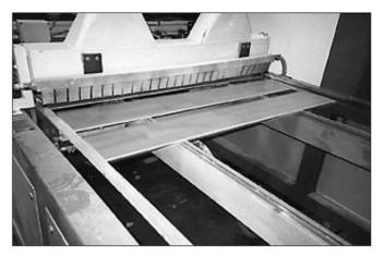
ALSAPAN in France uses an efficient custom manifold (Silvent 380 special, 40x40 aluminum profile – see reverse side of page) with flat nozzles to blow parquet blocks clean before varnishing.
