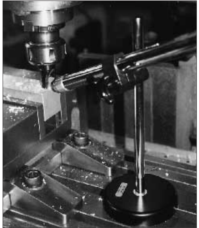
A Silvent 296 being used to keep the milling machine clean during operation. A knob and single-handed grip allow easy adjustment to the quietest and most efficient blowing angle.
