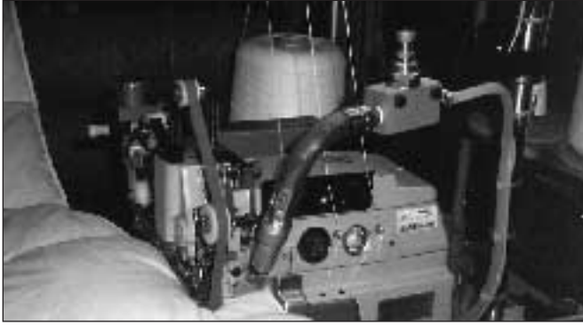
Textile industry. A Silvent 220 is used to keep the machine clean and avoid stoppage. Previously, a 4 mm open pipe was used. Switching to the 220 cut the noise level in half and reduced air consumption by 36%.
