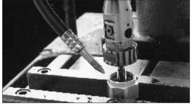
An Silvent 640 being used for cooling and cleaning in a tapping operation.
