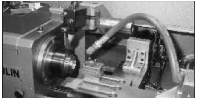
A flexblow hose and a Silvent nozzle - a very quiet and efficient combination for turning operations.
