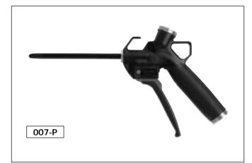
Silvent 007-P with its PEEK nozzle prevents unnecessary scratching. The PEEK nozzle has been specially developed for sensitive applications where expensive tools and machines absolutely may not be damaged. The nozzle is fitted on a flexible PA 12 pipe that provides additional protection against scratches caused by mechanical impact.
