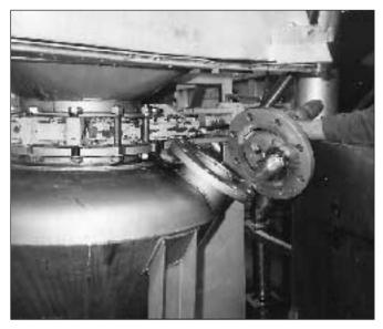
In this application Silvent's largest nozzle, the 720, blows a filet machine free of fish scraps. The Silvent installation replaced an open pipe that generated a noise level of 102 dB(A). The 720 has lowered the noise level to 79 dB (A) and provides a blowing force that is more than sufficient.
