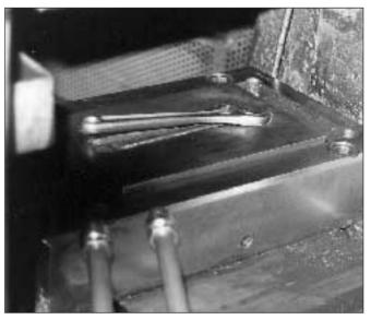
THE MANUFACTURING INDUSTRY. Sandvik Bahco uses 2 Silvent 705s to lift a 1 kilo crescent wrench off the die of a press. Previously 10 mm open pipe was used. By installing Silvent nozzles the noise level has been halved and, at the same time, air consumption has been reduced by 49%. At a degree of utilization of 40%, that means a cost savings of more than 850 USD per year.
