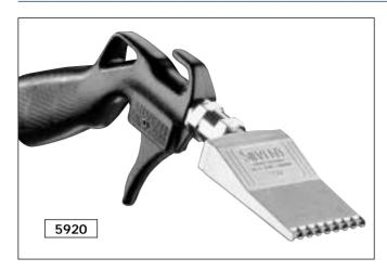
Silvent 5920 is an air gun with a flat nozzle for applications where you want the air stream to strike a wider surface, providing quick and efficient blow-off. This low-noise nozzle is made of zinc and its outlet ports are protected against external forces by fins. Patented.
