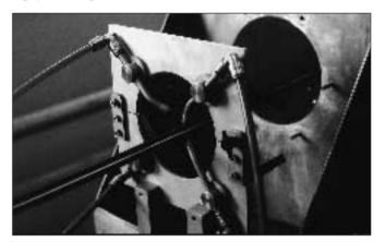
The picture shows four Silvent 5001 nozzles mounted around a plastic strip puller. The nozzles blow the plastic strip dry of water during continuous production. The company has confirmed that air consumption has decreased significantly and that the noise level has been reduced by 20% since switching from "open-pipe blowing".
