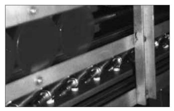
The picture shows a packaging machine that is equipped with 25 511s. The nozzles transport mustard lids. The noise level at the machines has been more than halved.
