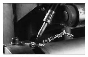
Blow-off at a lathe with a FLEXBLOW hose and a 511 nozzle.
