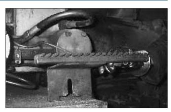
Blow-off after welding. One of the largest wheel rim manufactures in Europe, Prins Dokkum in Holland, uses Silvent's blowing nozzles in a number of different blowing operations. Here, an air bar with Silvent 511 nozzles. The bar is used for blowing away scale and debris following spot welding.
