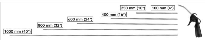
The 500 series is available with six different extension pipe lengths. The pipes are made of zinc-plated steel. Other materials and lengths can be supplied upon request. When ordering air guns with longer extension pipes than the standard 100 mm, specify the length you want last in the order number – pistol grip-nozzle-extension pipe length, e.g. 500-Z-600.
