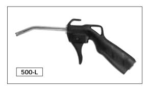
SILVENT 500-L has a stainless steel Laval nozzle. A Laval hole in the center of the nozzle creates a highly concentrated air stream that moves at supersonic speed. Around the Laval hole there are also a number of diverging slots that generate a powerful, quiet and laminar air flow. The combination provides superior cleaning performance and optimal utilization of the compressed air. The surrounding fins prevent direct contact between skin and the outlet holes. Patented.
