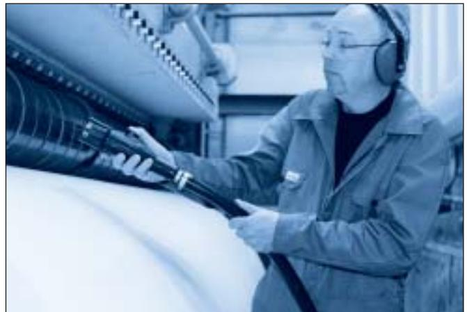
SILVENT4015-L with "dead man's grip" is used to safely clean a roller. Dead man's grip means that the valve will close instantly if the operator should drop the handle.
