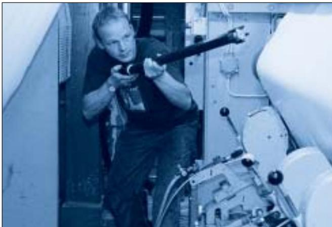
The picture shows a cleaning application at a paper mill. A 4015-LF-1000 is used to allow the operator to work with a more ergonomic posture and still reach deep into the machine.
