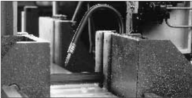
The picture shows a flexblow hose keeping a crosscut saw clean.
