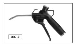
SILVENT 007-Z features a zinc slot nozzle designed with divergent slots that utilizes the surrounding air very efficiently. This nozzle allows powerful, quiet and efficient cleaning. Suitable for general-purpose blowing in environments where the nozzle is exposed to minimal mechanical wear. Patented.
