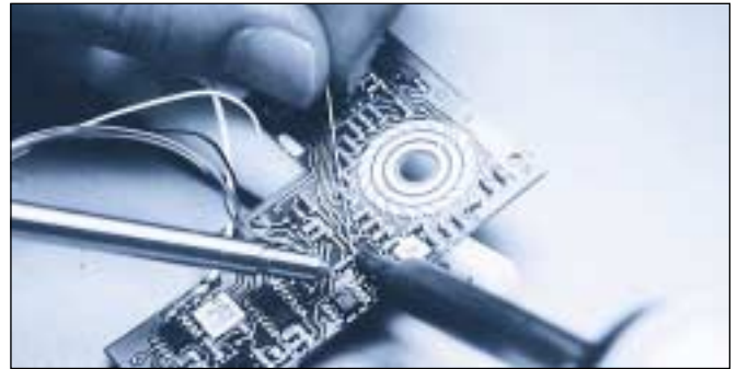
The picture shows an application where Silvent MJ6 is used for spot cooling and blow-off when soldering a printed circuit board.
