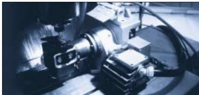
The picture shows an air knife blowing clean at a CNC machine used for machining the side piece of a camera housing at Hasselblad.
